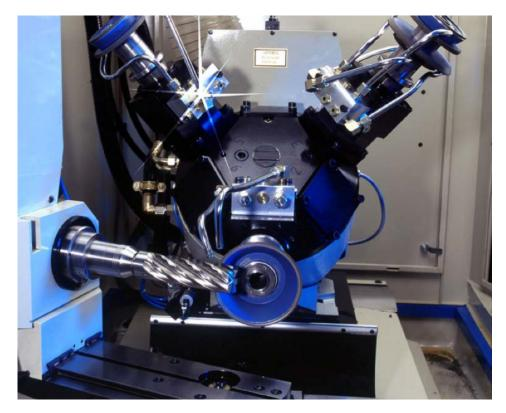
The multi spindle wheel head on the TG 600 CNC with 3 spindles (optional up to 6 spindles) makes grinding of complex tools, where several wheels are need, very easy. Since up to 6 wheel packages with 3-4 grinding wheels on each can be mounted at a time most type of tools can be ground without the need for wheel setup.
